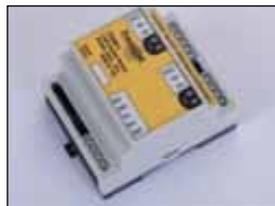
The instrumentation (TTSIM-1) provides excitation voltage that attempts to drive current from one electrode wire to the other every few seconds. No current flow is possible until an acid leak occurs.
