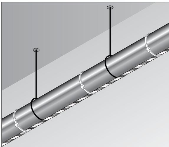
TT7000-HUV sensing cables are primarily intended for use on overhead piping, vertical pipe, valves and manifolds and other fittings where concentrated sulfuric or nitric acid could leak. Sensing cables can also be used on floors, in drip pans, in sumps, trenches and underground in slotted conduit. They may be pulled into double wall containment pipes or tanks to monitor interstitial space.
