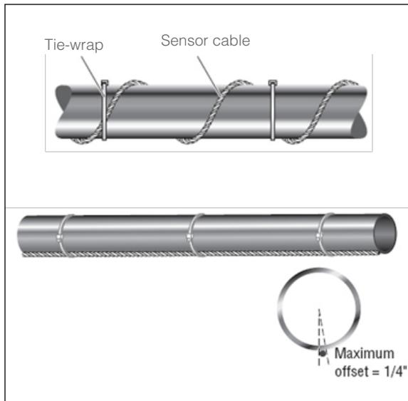
**Configurations for vertical and horizontal piping**
