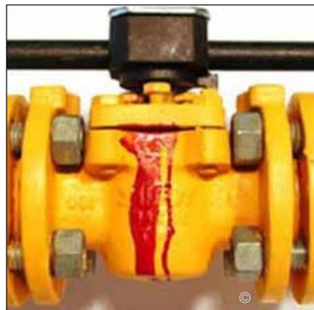
**Leak detection paint can be effective for use in in-line inspection**
