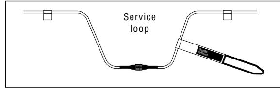
For sumps, containment trenches, and subfloor applications, a service loop should be provided at each cable connector.
